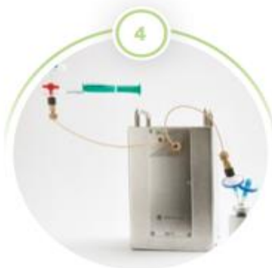
Elute the generator with 5 mL directly into vial 1.
