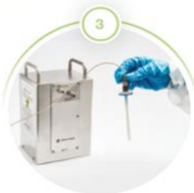
Assemble sterilizing filter between outlet line and sterile needle. Check the luer lock connection before elution.
